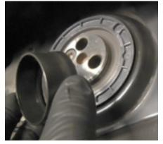
5 With the specific tool, turn clockwise for the final fitting of the seal with the cover.
