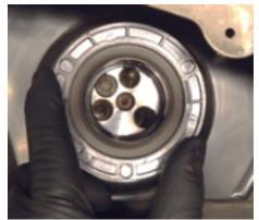
4 Push uniformly the seal towards the cover to fit the seal on the cover and over the shaft and then
